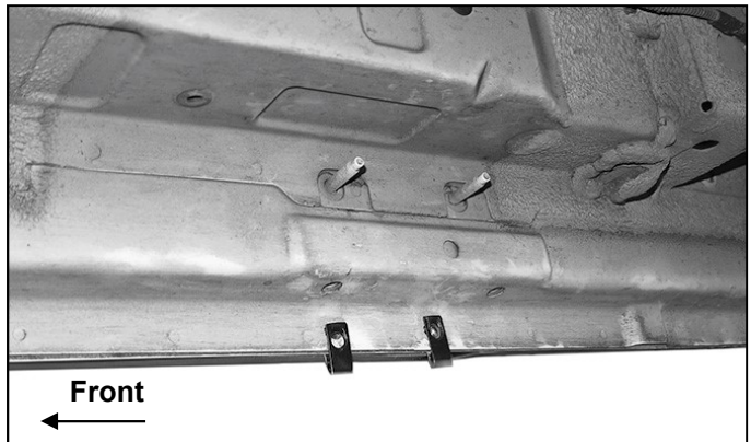
(Fig 10) Remove Bracket. Slide 8mm Clip Nuts onto pinch weld and over drilled holes. NOTE: 8mm U-Bolt is not required on mounting location with factory mounting studs (rear location pictured)
